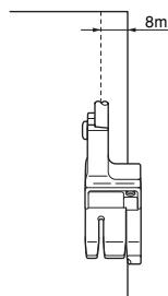
1. Fold the seam allowance to one side, and then sew topstitching while aligning the guide with the edge of the fold.
