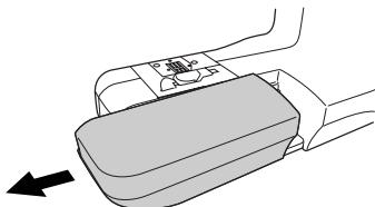
With the flat bed attachment removed, free-arm sewing is possible.
