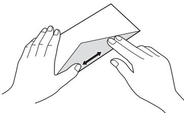
Fan the stack of envelopes well to avoid paper jams and misfeeds.
