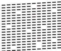
6. The LCD asks you to check the print quality of each colour. Press **◀** or **▶** to select the pattern (1–4) that most closely matches the printing result, and then press **OK**.
