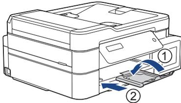
2. Pull the paper tray completely out of the machine.
