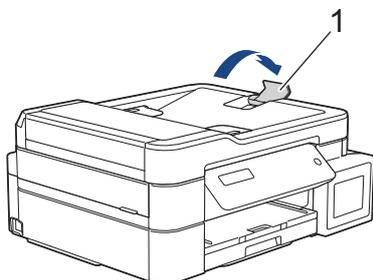
2. Fan the stack of paper well to avoid paper jams and misfeeds.
