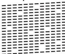
6. The LCD asks you to check the print quality of each colour. Press **▲** or **▼** to select one of the patterns that most closely matches the printing result, and then press **OK**.
