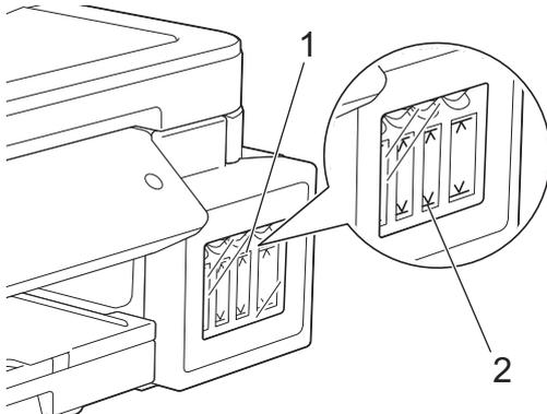
The ink below the lower line is necessary to prevent air from drying out and damaging the print head assembly. Refill the ink tank when the remaining ink level is at or below the lower line.
