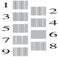
5. For pattern (A), press **◀** or **▶** to select the number of the test print that has the fewest visible vertical stripes (1-9), and then press **OK**.
