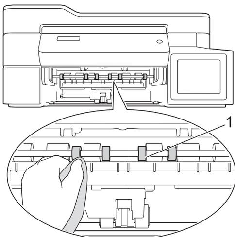
5. (MFC-T910DW) Lift the Jam Clear Flap (2), and then clean the back side of the Paper Feed Rollers (1) with a soft lint-free cloth moistened with water. After cleaning, wipe the rollers with a dry, soft lint-free cloth to remove all moisture.
