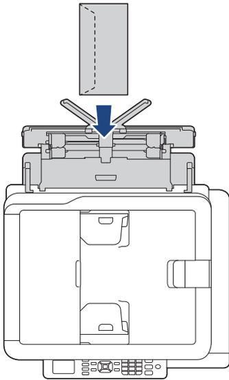
If you are having difficulty loading paper in the MP tray, push the release lever (1) towards the back of the machine, and then load the paper.
