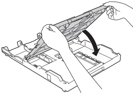
6. Load up to 20 sheets of photo paper with the printing surface **face down**.
