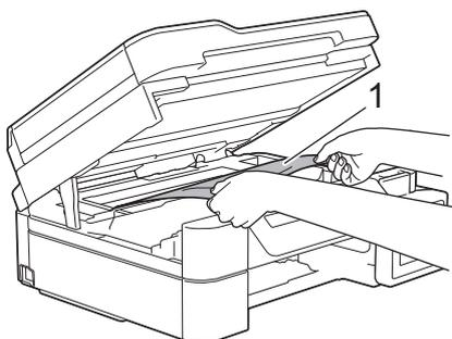
6. Move the print head (if needed) to take out any paper remaining in this area. Make sure scraps of paper are not left in the corners of the machine (1) and (2).
