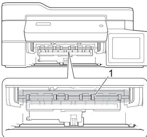
10. Squeeze both levers (1), and then open the Jam Clear Cover at the back of the machine.
