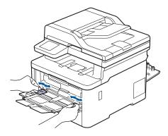
6. Load paper with the printing surface face up in the MP tray.
