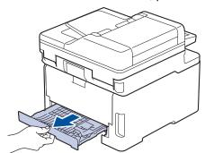
4. Pull the jammed paper out of the machine or out of the 2-sided tray.
