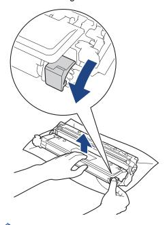
To avoid print quality problems, DO NOT touch any surface of the drum unit except the drum unit gear.
