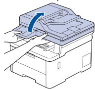
• You can still use the machine while the scanner cover is up. To close the scanner cover, gently push it down with both hands.
