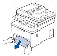
Pulling the jammed paper downwards using both hands allows you to remove the paper more easily.
