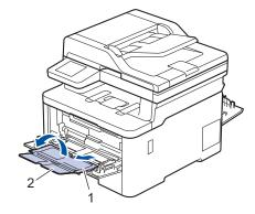
4. Slide the MP tray paper guides to fit the width of the paper you are using.
