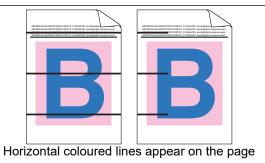
Identify the colour causing the problem and replace the toner cartridge that matches the colour of the line.
