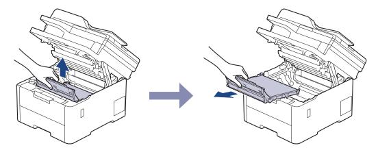
5. Unpack the new belt unit and insert it into the machine.
