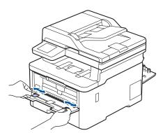
4. Using both hands, place one sheet of label in the manual feed slot until the front edge touches the paper feed roller. When you feel the machine pull it in, let go.
